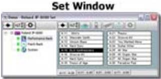
Sets contain structured 'snapshots' of your instrument's memory. Step between and edit each component.
